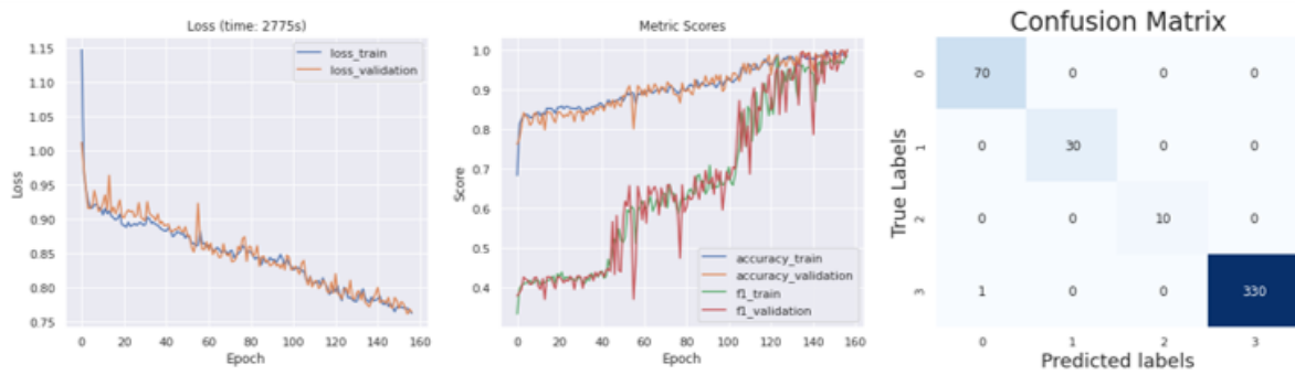
Figure 6.10: The loss curve (left), performance metrics (middle) and confusion matrix (right) for the InceptionTime model trained on the Hydraulic dataset.
